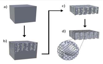
Fig. 1 Schematic of sample preparation process: (a) p-doped bulk silicon, (b) mesoporous silicon on bulk silicon after electrochemical etching, (c) free-standing mesoporous silicon membrane detached from mother substrate, (d) graphene-mesoporous silicon nanocomposites.
