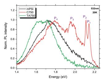
Fig. 7 PL spectra of three different samples: a mPSi film, a thermally annealed mPSi film (TA750), and a GPSi-nCs film produced at 750 °C (C750). For the C750 sample, the designated  $P_1$ ,  $P_2$ ,  $P_3$  and  $P_4$  emission bands are common for each of our graphene-coated film.
