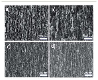
Fig. 2 Scanning electron microscopy (SEM) cross section images: (a) mPSi membrane, (b) thermally annealed mPSi at 750  $^{\circ}$ C (TA750), (c) GPSi-nC formed at 750  $^{\circ}$ C (C750), (d) GPSi-nCs formed at 850  $^{\circ}$ C (C850).
