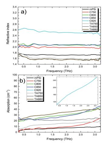
Fig. 5 (a) Refractive index of samples increasing with graphene deposition temperature. (b) Evolution of the samples absorption coefficient with frequency. The low mPSi absorption coefficient (<10 cm<sup>-1</sup>) within 0.3-3 THz range is consistent with literature.<sup>10</sup> The absorption level increases with graphene deposition temperature.
