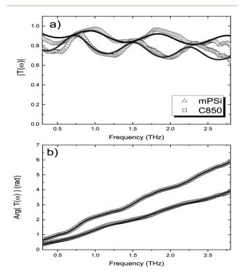
Fig. 4 Amplitude (a) and phase (b) of the complex transfer function. The solid lines correspond to the best fits to the data using eqn (1) and (2).
