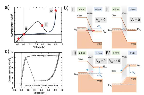
Fig. 1 (a) J-V characteristic of an ideal tunneling diode (full line) compared with a standard p-n diode (dashed). (b) Band diagram of the tunneling diode with degenerate doping of the p-type and n-type semiconductors, under different polarization conditions (I–IV). Red arrow: Electron field-emission current, blue arrow: electron diffusion current. Adapted from ref. 18. (c) Experimental J-V curve of a tunneling diode composed of a degenerate doped GaAs junction. Panel (b) adapted from ref. 20.
