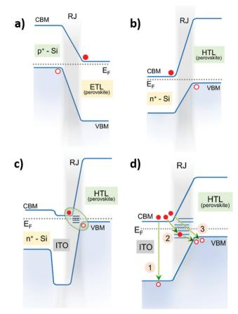
Fig. 2 Band diagrams of the RJ in silicon/perovskite tandems. (a) and (b) General cases of p-i-n and n-i-p tandems based on the perovskite top cell configuration. (c) Band diagram of the ITO-assisted RJ. (d) Zoom-in of panel c that represents the recombination mechanisms at the ITO/perovskite HTL interface for a p-i-n tandem
