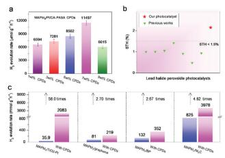
**Fig. 4** Efficiency optimization and performance comparison of CA-PASA CPDs with other electron-transfer materials. (a) Rate of  $H_2$  evolution on Pt/ MAPbl $_3$ /CA-PASA CPDs with different CPD contents. (b) STH conversion efficiencies of previous MHP photocatalysts.  $^{10,13,15-17,23-25,37,38,41-44}$  (c) Rate of  $H_2$  evolution on MAPbl $_3$ /TiO $_2$ -Pt, MAPbl $_3$ /graphene, MAPbl $_3$ /BP, MAPbl $_3$ /Ni $_3$ C, and their CA-PASA CPD-hybrid systems.
