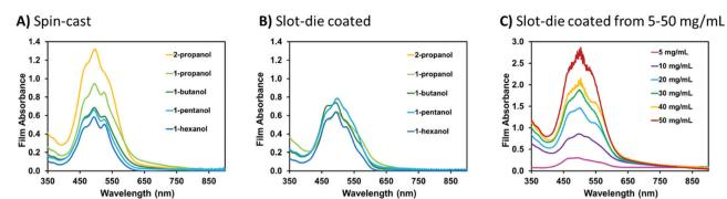
Fig. 5 Optical absorption spectra of (A) PDIN-H films spin-coated from different alcohols at 10 mg mL<sup>-1</sup>, (B) PDIN-H films slot-die coated from different alcohols at 10 mg mL<sup>-1</sup>, and (C) PDIN-H films slot-die coated from 1-propranol at varying concentrations onto PET. In all cases 1 molar equivalent NaOH was added to each pre-deposition solution.
