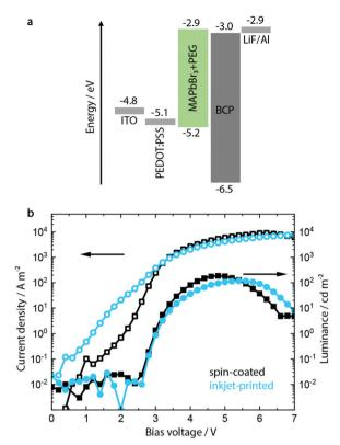
Fig. 1 (a) The energy levels of the chosen perovskite light-emitting diode (PeLED) device architecture permit ohmic contact between both the hole and electron injection layer and the semiconducting perovskite. (b) Current density/voltage/luminance characteristics show similar device parameters for the spin-coated and inkjet-printed PeLEDs without KCl as additive.
