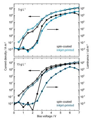
**Fig. 4** The J/V/L characteristics of PeLEDs fabricated on PEDOT:PSS blended with a low 5 g L $^{-1}$  KCl content (a) and high 15 g L $^{-1}$  KCl content (b) indicate the two different optimums depending on the process – for low KCl content devices incorporating the inkjet-printed active layer outperform those incorporating the spin-coated ones. For higher KCl content, it is *vice versa*.
