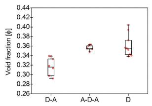
Fig. 3 Calculated void fractions  $\varphi$  for the three family molecules studied in this work and listed in Table 1. The box plot denotes median (centre line), 25th quartile (bottom edge of the box), 75th quartile (top edge of the box), maximum and minimum values. Only non-solvated structures have been considered
