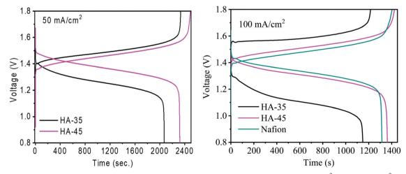
Charging and discharging for single cell VRFB with HA-35, HA-45 and Nafion 117 membrane at 50 mA cm $^{-2}$  and 100 mA cm $^{-2}$  current density.
