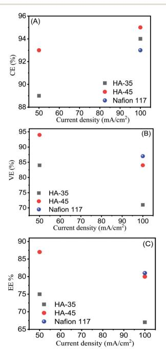
**Fig. 5** Coulombic, voltage and energy efficiencies *vs.* current density for HA-35, HA-45 and Nafion 117 membranes.
