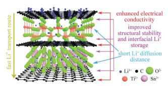
Fig. 8 A schematic illustration of the lithium ion storage mechanism in the SnO<sub>2</sub>@TiO<sub>2</sub>/C nanoarchitecture.
