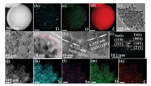
Fig. 3 (a) High angle annular dark field image and the corresponding EDS elemental mapping images of Ti (b), O (c), and C (d) of TiO<sub>2</sub>/C spheres; (e) TEM image of crushed TiO2/C spheres; (f) TEM image, (g and h) HRTEM image, and (i) the corresponding SAED pattern of SnO2@TiO2/C; and (j) HAADF image and the corresponding EDS elemental mapping images of Ti (k), Sn (l), O (m), and C (n) of  $SnO_2@TiO_2/C$
