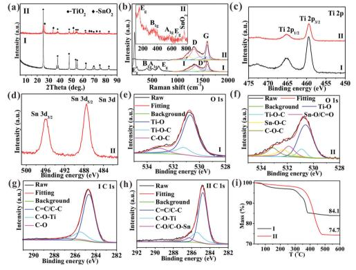
Fig. 2 (a) XRD, (b) Raman spectra, (c-h) XPS spectra of Ti 2p (c), Sn 3d (d), O 1s (e and f), and C 1s (g and h), and (i) TG curves of TiO<sub>2</sub>/C (I) and SnO<sub>2</sub>@TiO<sub>2</sub>/C (II).
