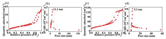
Nitrogen adsorption-desorption isotherms and pore-size distribution of TiO<sub>2</sub>/C (a and b) and SnO<sub>2</sub>@TiO<sub>2</sub>/C (c and d).
