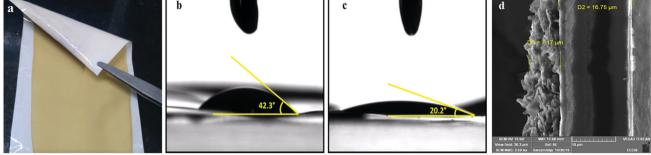
Fig. 2 (a) Digital photograph of the POP coated 2320-type Celgard membrane, contact angle shots of (b) CG 2320 and (c) POP-CG and (d) the crosssectional SEM image of the POP coated Celgard membrane.
