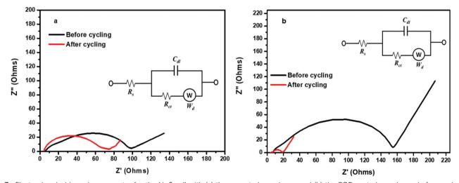
Fig. 7 Electrochemical impedance spectra for the Li–S cell with (a) the uncoated membrane and (b) the POP coated membrane before and after cycling. Inset: The corresponding equivalent circuits.
