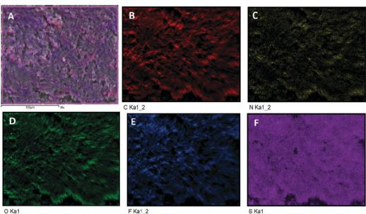
Fig. 8 Panel (1): the EDS spectrum of the POP coated membrane after cycling; panel 2 and 3: (A) the FE-SEM image of the POP coated membrane and elemental mapping of (B) carbon, (C) nitrogen, (D) oxygen, (E) fluorine and (F) sulfur after cycling.
