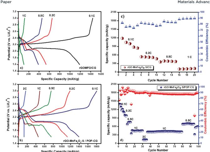
Fig. 5 Charge-discharge curves of the Li-S cell with (a) Celgard and (b) POP-coated CG membranes and discharge capacity vs. cycle number of the Li-S cell at different C-rates (c) with Celgard and (d) POP-coated Celgard membranes
