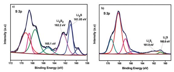
XPS detailed scans of the Li anode surface (a) with CG 2320 and (b) POP-CG after cycling. Fig. 9
