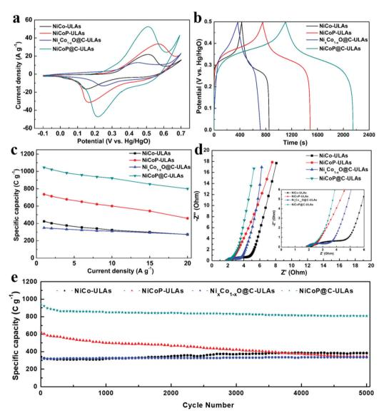
Fig. 8 Electrochemical performances of different electrodes. (a) CV curves at a scan rate of 10 mV s $^{-1}$ , (b) GCD curves at a current density of 1 A g $^{-1}$ , (c) specific capacity at different current densities. (d) Nyquist plots; the inset shows the high-frequency region. (e) Cycling performance at a constant current density of 8 A g $^{-1}$ .
