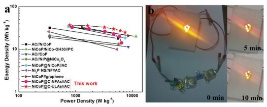
Fig. 10 (a) Ragone plots of the NiCoP@C-ULAs//AC, NiCoP@C-NFAs//AC and reported Ni or Co-based ASC devices; (b) optical images of six LEDs lit up by NiCoP@C-ULAs//AC devices.
