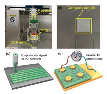
Fig. 1 Alignment of  $BaTiO_3$  nanowires in nanocomposites: photographs of (a) the printing assembly and (b) a printed nanocomposite sample; schematic illustrations of (c) the alignment of  $BaTiO_3$  nanowires in the P(VDF-CTFE) matrix and (d) a nanocomposite capacitor for energy storage applications.
