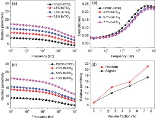
Fig. 4 Frequency dependence of (a) relative dielectric permittivity and (b) dielectric loss of BaTiO<sub>3</sub>/P(VDF-CTFE) nanocomposites with aligned BaTiO<sub>3</sub> nanowires. (c) relative dielectric permittivity of nanocomposites with random distributed BaTiO<sub>3</sub> nanowires; (d) relative dielectric permittivity of the nanocomposites as a function of volume fraction at 1 kHz.
