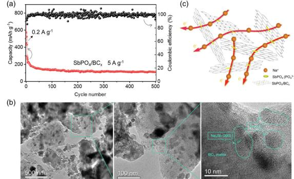
Fig. 6 (a) Cycling performance of the SbPO<sub>4</sub>/BC<sub>y</sub> electrode at 5 A  $q^{-1}$  after three cycles at 0.2 A  $q^{-1}$ . (b) TEM images of the SbPO<sub>4</sub>/BC<sub>y</sub> electrode after 500 cycles. (c) Proposed mechanism of the SbPO<sub>4</sub>/BC<sub>x</sub> composite during the sodium storage processes
