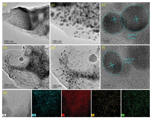
Fig. 2 TEM images (a and b) and HRTEM images (c) of the Sb/ BC<sub>x</sub> composite; TEM images (d and e) and HRTEM images (f) of the Sb/C composite; (g) scanning TEM image with its corresponding EDS mappings of the Sb, C, B and O elements for the Sb/BC $_x$  composite.
