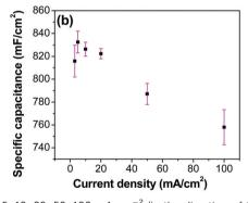
Fig. 9 (a) GCD curves for  $RuO_2$ -CNF prepared at 250 °C, recorded at 3, 5, 10, 20, 50, 100 mA cm<sup>-2</sup> (in the direction of the arrow, respectively). (b) Variation of specific capacitance with the change in current density calculated from the GCD measurements.
