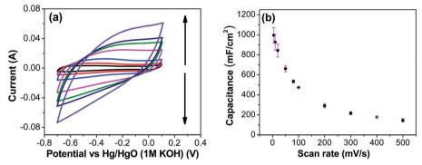
Fig. 13 (a) CV curves of  $RuO_2$ -CNF prepared at 250 °C recorded in a three-electrode cell at scan rates of 5, 10, 20, 50, 80, 100, 200 mV s<sup>-1</sup> (the scan rate increases in the direction of the arrows). (b) Change in capacitances with scan-rate (capacitance values are reported per electrode).
