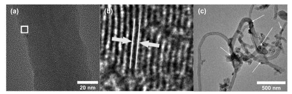
Fig. 3 (a) HR-TEM image of uncoated CNF showing a large number of zones having graphitic layer structures when viewed in high resolution, (b) enlarged image of the white-box in Fig. 3b, showing one example of such zone. The white lines and the arrow depict the spacing between the graphitic layers, which is found to be ca. 0.34 nm, characteristic of graphite. (c) TEM image of RuO<sub>2</sub>-CNF electrode prepared at 250 °C. Arrows show some RuO<sub>2</sub> sheets (dark regions).
