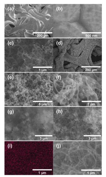
Fig. 2 SEM images of (a and b) Ni-f before the growth of CNF, and (c) uncoated CNF. (d-f) Secondary electron images recorded at different magnifications, (g and h) BSE and the corresponding SE image of RuO<sub>2</sub>-CNF prepared at 250 °C (i and j) EDX map showing the distribution of elemental ruthenium and the corresponding SE image of RuO2-CNF prepared at 250 °C, respectively
