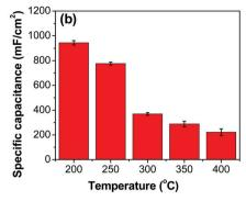
Fig. 6 (a) CV measurements of  $RuO_2$ -CNF electrodes prepared at different temperatures, recorded in a two-electrode setup at 20 mV s<sup>-1</sup>. (b) Specific capacitances determined from CV curves.
