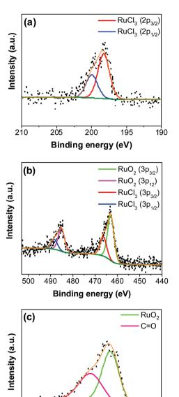
Fig. 5 Fitted HR-XPS of the RuO<sub>2</sub>-CNF electrode surface prepared at 250  $^{\circ}\text{C}$  (a) Cl 2p, (b) Ru 3p, and (d) O 1s. Black dots, olive and orange line represents, experimental data, background and fitted data respectively.
