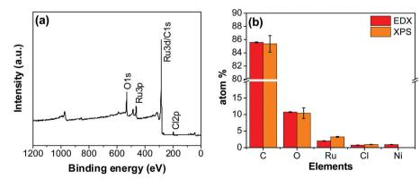
Fig. 4 (a) XPS survey scan of the RuO<sub>2</sub>-CNF electrode prepared at 250 °C. (b) The elemental composition of the RuO<sub>2</sub>-CNF electrode determined using EDX and XPS. n = 3.
