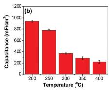
Fig. 10 (a) Nyquist plots for RuO<sub>2</sub>-CNF electrodes prepared at different temperatures (inset: the zoomed-in high-frequency region). The spectra were recorded at cell potential of 0 V (b) capacitance values obtained from EIS measurements for electrodes prepared at different temperatures.
