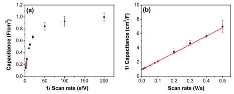
Fig. 14 (a) Capacitance as a function of the inverse of scan rate for the  $RuO_2$ -CNF electrodes prepared at 250 °C. (b) The inverse of capacitance as a function of scan rate. Red line indicates linear fit with the equation (a) y = 0.05x + 0.06, and (b) y = 11.76x + 0.94.
