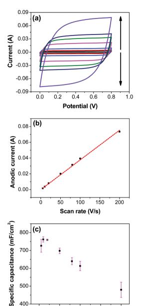
Fig. 7 (a) CV of RuO2-CNF electrodes prepared at 250 °C recorded at scan rates of 5, 10, 20, 50, 80, 100, 200 mV  $s^{-1}$  (the scan rate follows the direction of the arrows). (b) Corresponding anodic current determined at a potential of 0.5 V as a function of scan rate. Red-dotted line is linear fit with the equation of  $y = 3.76 \times 10^{-4} x$ . (c) Variation of the specific capacitance with scan rate calculated from the CV measurements.
