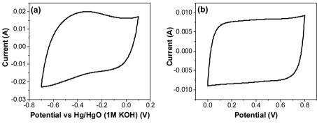
Fig. 12 CV of RuO<sub>2</sub>–CNF electrodes prepared at 250  $^{\circ}$ C, in 6 M KOH electrolyte recorded at 20 mV s<sup>-1</sup> (a) using a three-electrode cell, and (b) using a two-electrode cell.
