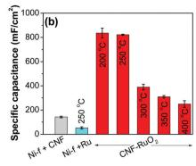
Fig. 8 (a) GCD plots recorded at 20 mA cm $^{-2}$  for Ni-f-RuO<sub>2</sub> (red), Ni-f-CNF (black), and RuO<sub>2</sub>-CNF electrodes prepared at 400, 350, 300, 250, and 200 °C (in the direction of the arrow, respectively). (b) Corresponding specific capacitance values.
