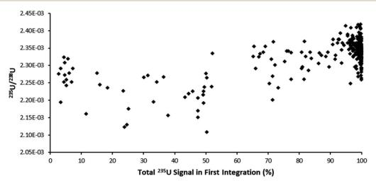
Fig. 5 Plot of  $^{235}$ U/ $^{238}$ U for single-shot laser ablation pulses on SRM611, integration time 262 ms, against the percentage of  $^{235}$ U signal contained within the first integration. Pulses with 100% of the  $^{235}$ U signal in a single integration were biased higher relative to pulses split between two integrations.
