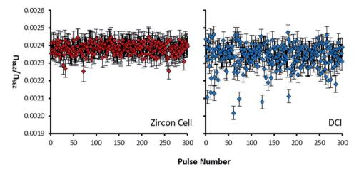
Fig. 3  $^{235}$ U/ $^{238}$ U isotope ratios of 300 pulses on SRM611 glass, calculated by total signal integration. Plot on the left (red) is for the Zircon Cell, plot on the right (blue) the DCI. Error bars on each ratio are 2SE, determined from counting statistics. All of the pulses collected with the Zircon Cell describe a single population within 2SD. Some pulses collected with the DCI had depleted  $^{235}$ U/ $^{238}$ U values, out with uncertainty, relative to the main population.
