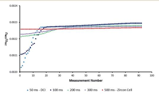
Fig. 6 Plot of possible uncorrected  $^{235}$ U/ $^{238}$ U isotope ratios for the average model pulse due to the influence of blind time. The 100–300 ms datasets were created by widening the model IC pulse *via* changes to the parameters in the exponential-Gaussian hybrid function. As the pulse duration increased, the impact of blind time on isotope ratio accuracy was reduced.
