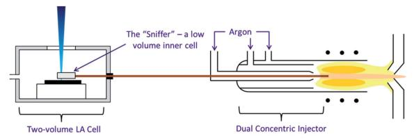
Fig. 1 The three components of the high speed, integrated ablation cell and DCI, reproduction from Douqlas D. N., Managh A. J., Reid H. J., Sharp B. L., Anal. Chem., 2015, 87(22), 11285-11294.
