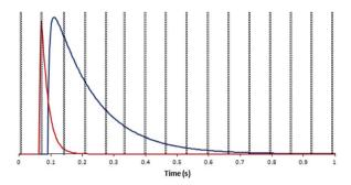
Fig. 4 Model <sup>235</sup>U IC signal response (red) and <sup>238</sup>U Faraday detector signal response (blue) for the DCI: created with the determined exponential Gaussian hybrid functions, values every 3 ms. Blind time events (black dotted box) denote an example 66 ms integration time. The proportion of total counts lost to blind time differs between the IC and Faraday signal responses.
