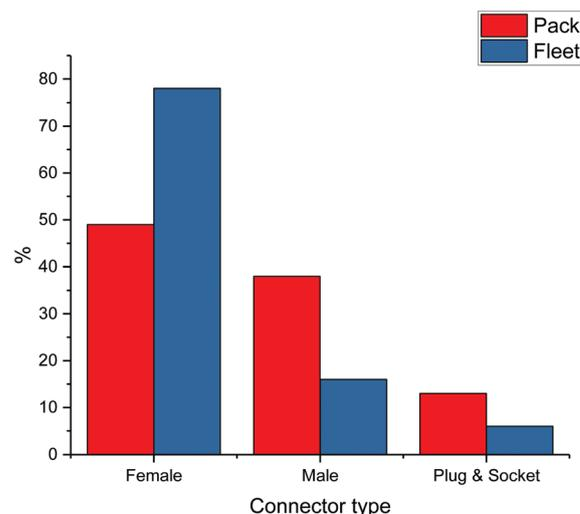
**Fig. 9** (red) Proportion of packs utilising each intermodular connection type, (blue) proportion of connection type across fleet population of modules. Data from 2018 EU sales of (H)EVs where available.
