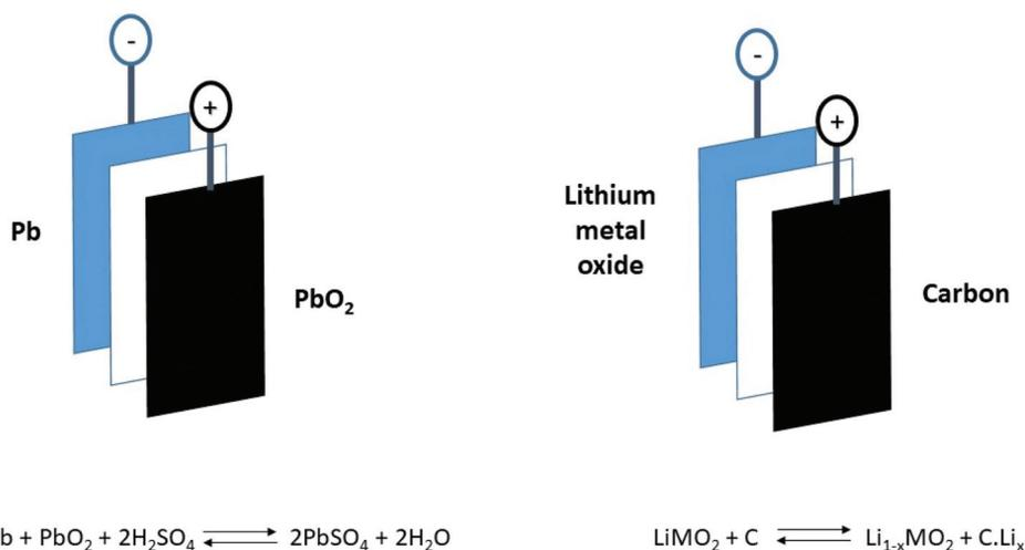
Fig. 1 Basic schematic of a lead acid and lithium ion battery.<sup>6</sup>
