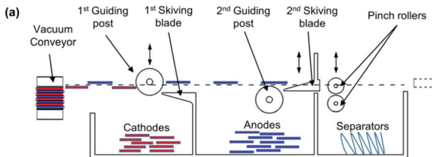
**Fig. 6** Schematic diagram of a prototype device for separating anodes, cathodes and separators from a lithium ion battery.<sup>42</sup>
