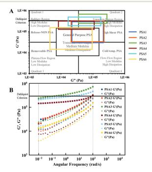
**Fig. 3** (A) Chang's viscoelastic window of pressure-sensitive adhesives applied to the synthesised PSAs and (B) frequency sweep measurements performed at room temperature by rheology.
