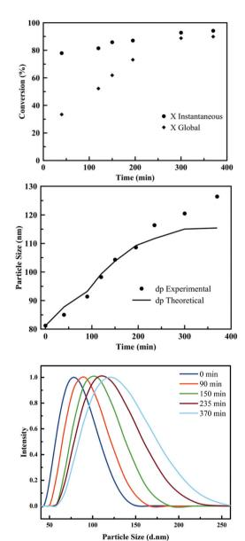
Fig. 2 The conversion as a function of time (top), the evolution of the particle size as a function of time (middle) and the corresponding DLS traces (bottom) of PSA2 during feeding in the seeded semi-batch emulsion polymerization.
