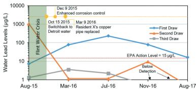
Fig. 3 Water lead levels (first draw, second draw, and third draw) in five sampling rounds during 2015–17 for resident X, who had a copper service line that was removed and replaced with a new copper pipe on March 9, 2016.
