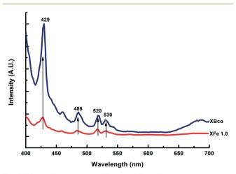
Fig. 6 PL emission spectra of XBco and XFe-1.0
