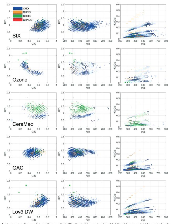
Fig. 2 Van Krevelen diagrams (left panel), mass edited H/C ratios (middle panel) and modified Kendrick mass plots (right panel) of molecular compositions that decreased in relative abundance by more than 50% after each pilot treatment process. Comparisons were made for compositions detected in three replicates with final water from the conventional treatment at Lovö used as a reference (Lovö DW).
