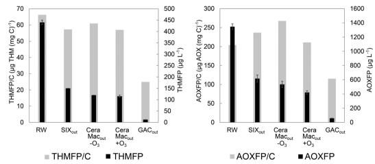
Fig. 6 THM formation potential (THMFP), AOX formation potential (AOXFP), THM formation potential per mg carbon (THMFP/C) and AOX formation potential per mg carbon (AOXFP/C) upon chlorination ( $\sim$ 10 mg L $^{-1}$  chlorine residual) at different stages of the pilot treatment (RW, SIX<sub>out</sub>, CeraMac<sub>out</sub> - O<sub>3</sub>, CeraMac<sub>out</sub> + O<sub>3</sub>, GAC<sub>out</sub>) (experiment 3).
