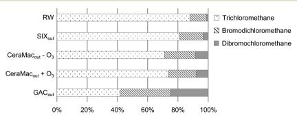
Fig. 7 Percentage of different THM species formed during high-dose chlorination after each stage of the pilot treatment (RW, SIX<sub>out</sub>, CeraMac<sub>out</sub> - O<sub>3</sub>, CeraMac<sub>out</sub> + O<sub>3</sub>, GAC<sub>out</sub>), based on the average of two replicates (experiment 3). Tribromomethane was not detected.
