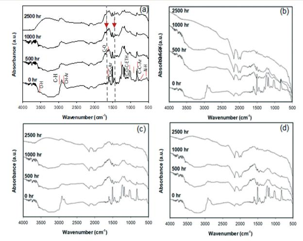
Fig. 1 ATR-FTIR spectra of (a) neat epoxy, (b) epoxy-CB, (c) epoxy-CNT, and (d) epoxy-GP composites, after 0, 500, 1000, and 2500 h of wet weathering (arrows show absorption peaks used to calculate the CI).
