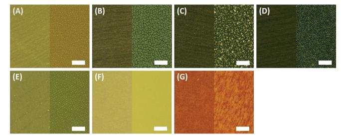
Fig. 2 Optical images (250×) of surfaces of: (A) unfilled epoxy, (B) epoxy-carbon black composite, (C) epoxy-graphene composite, (D) epoxy-MWCNT composite, (E) epoxy-SiO<sub>2</sub> composite, (F) unfilled polypropylene, (G) PP-Fe<sub>2</sub>O<sub>3</sub>. The left half of each image shows un-weathered sample and the right half shows samples weathered for 2500 h in an accelerated wet weathering chamber. Scale bar is 250  $\mu$ m for all images.
