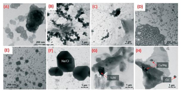
Fig. 7 A selection of TEM pictures of debris present in the leachates of PA wafers. In the first row, PA wafers were aged (A and B) 0 h and (C and D) 2500 h in the second row, PA-kaolin wafers were weathered (E and F) 0 h and (G and H) 1000 h.
