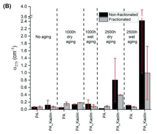
Fig. 5 Absorption coefficient measurements at 275 nm ( $\alpha_{275}$ ) of leaching fluids from (A) epoxy and (B) PA samples, resulting from different aging (time, wet/dry) and fractionation (fractionated/nonfractionated) protocols. Wet-aged samples were averaged between laboratories. Dry-aged samples were aged and analyzed by BASF only.
