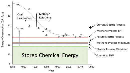
Fig. 3 Improvement in the efficiency of ammonia production over the last decades showing actual plant data compared to Best Available Technique (BAT), the minimum energy requirement for a methane-fed plant, the minimum energy for electrolysis (H<sub>2</sub> LHV), and current and future electrically driven processes. The amount of energy stored in ammonia is the lower heating value (LHV) and everything above that is losses. Data points acquired from ref. 33 and 34.
