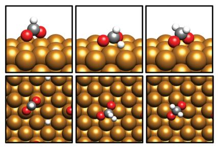
Fig. 9 Graphic depicting shift from O coordination from on-top to bridging Cu sites during hydrogenation from HCOO\* to H₂COO\* over Cu(100). The initial (left), transition state (middle) and final (right) geometries are depicted from the side (top) and from above (bottom).
