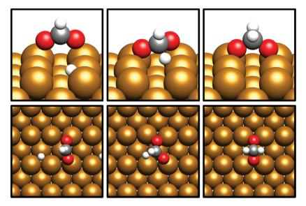
Fig. 8 Graphic depicting shift from O coordination from on-top to bridging Cu sites during hydrogenation from HCOO\* to  $H_2COO$ \* over Cu(110). The initial (left), transition state (middle) and final (right) geometries are depicted from the side (top) and from above (bottom). The "long bridge" adsorption geometry is shown as this is the most stable final state and yields the lowest activation barrier for  $H_2COO$ \* formation.
