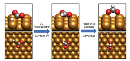
Fig. 5 Graphical depiction of hydrogenation of activated CO<sub>2</sub> to formate over Cu(110). The left panel shows the initial state geometry, the middle panel shows the monodentate species arising from C-H bond formation, and the right panel shows the most stable bidentate HCOO\* geometry. A side view is presented in the top half of each panel, whist the bottom half shows a view from above the Cu(110) slab.
