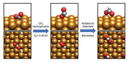
Fig. 6 Graphical depiction of hydrogenation of activated CO<sub>2</sub> to formate over Cu(100). The left panel shows the initial state geometry, the middle panel shows the monodentate species arising from C-H bond formation, and the right panel shows the most stable bidentate HCOO\* geometry. A side view is presented in the top half of each panel, whist the bottom half shows a view from above the Cu(100) slab.
