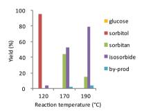
Fig. 3 Effect of reaction temperature at 24 h reaction time on the direct, catalytic conversion of glucose over bifunctional Ru@Dowex-H (0.2% w/w Ru, water, 30 bar H<sub>2</sub>). Adapted with permission from ref. 261. Copyright 2016, Royal Society of Chemistry.
