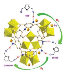
Scheme 13 Molecular interactions in the hydrogenation of HMF over Pd/ MIL-101(Al)-NH $_2$ . Gray and blue balls represent carbon and nitrogen atoms, respectively. The palladium nanoparticles are golden in color. Reprinted with permission from ref. 293. Copyright (2015) American Chemical Society.
