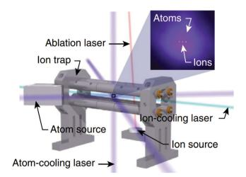
Fig. 4 Schematic depiction of a hybrid atom-ion trap. With careful alignment of the two trap centres, an ensemble of trapped ions can be spatially overlapped with a cloud of laser-cooled atoms. Reprinted from Schowalter et al., 121 under the terms of the Creative Commons CC BY license. Copyright 2016, Springer Nature.
