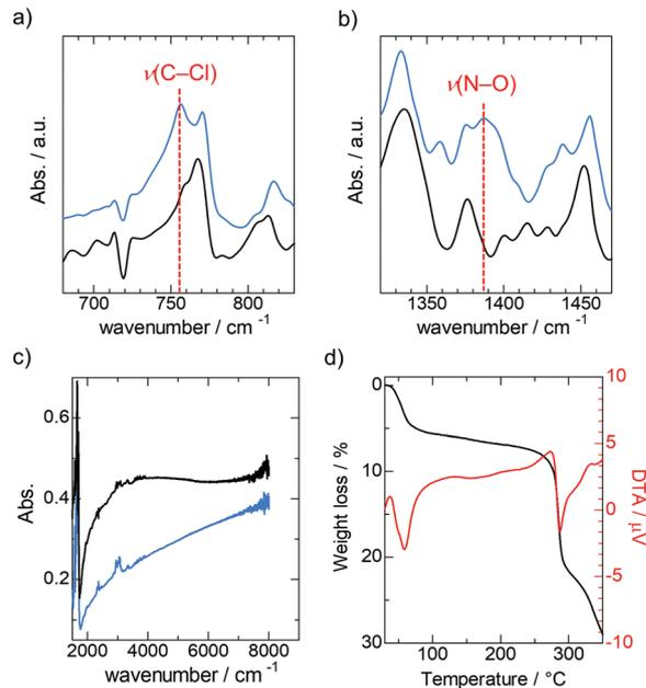
Fig. 4 (a–c) IR absorption spectra of **1** (blue) and **2** (black). The red dashed lines in (a) and (b) represent the reported absorption wavenumber for the C-Cl vibration mode (feature of chloroform) and N-O vibration mode (feature of  $\text{NO}_3^-$  ion), respectively. (d) TGA and DTA trace of **2**.
