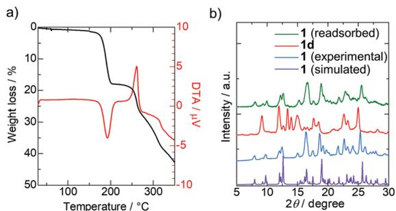
**Fig. 2** (a) TGA and DTA trace of **1**. (b) PXRD patterns of **1d** (red) and **1** (simulated from the crystal structure: purple, experimental: blue, after soaking **1d** in chloroform for a day: green).
