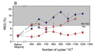
Fig. 4 Hydrodynamic performance of fatigued J6 valves. (A) Effective Orifice Area (EOA); (B) fractional regurgitation (REG). Error bars indicate variation between repeated measurements of the same valve.
