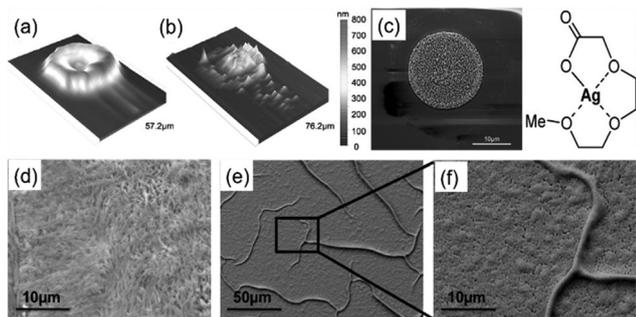
**Fig. 10** (a and b) The 3D profilometer image of an inkjet printed, dried and sintered (250 °C, 1 min) droplet of the silver(II) 2-[2-(2-methoxyethoxy)ethoxy]acetate ink; (c) SEM image of a sintered (250 °C, 1 min) droplet; (d–f) SEM images of the printed layer and sintered silver layer (5 min, 250 °C). Reproduced with permission from ref. 82. Copyright 2010, American Chemical Society.
