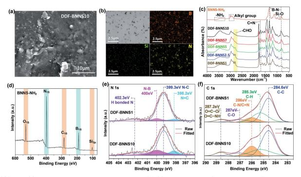
Fig. 1 (a) SEM and (b) TEM images and element mapping of DDF-BNNS10; (c) FTIR spectra of BNNS-NH2 and DDF-BNNS samples with different BNNS-NH2 content values; (d) the XPS spectrum of BNNS-NH2; and (e) N 1s core-level and (f) C 1s core-level spectra of DDF-BNNS1 and DDF-BNNS10.
