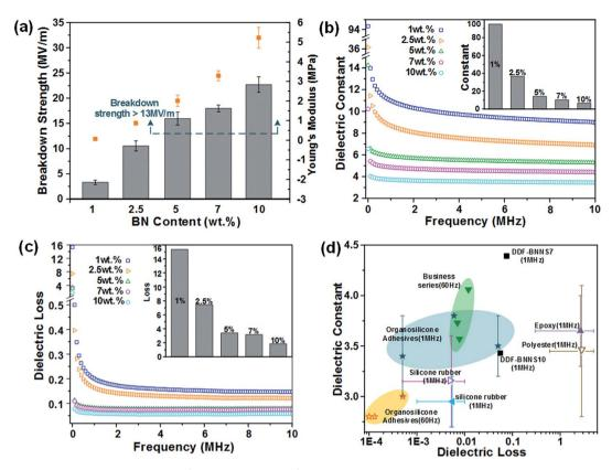
Fig. 4 (a) The breakdown strength of DDF-BNNS with different BNNS-NH<sub>2</sub> content. The frequency-dependent dielectric constant (b) and loss (c) of DDF-BNNS with different BNNS-NH<sub>2</sub> content; inset: dielectric constant (b) and loss (c) of DDF-BNNS with different BNNS-NH<sub>2</sub> content at 20 MHz. (d) A comparison of dielectric constant and loss values between different adhesives and insulating materials.
