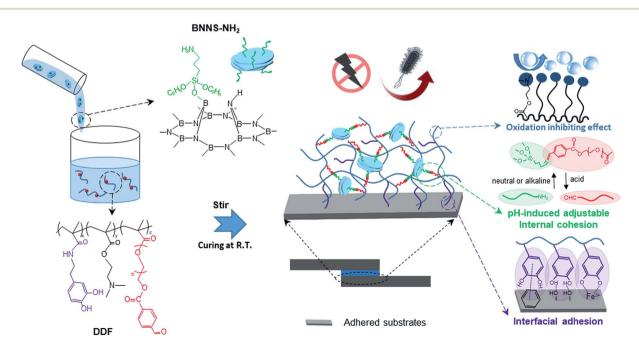
Scheme 1 The synthesis route of the NCA and its multiple characteristics (anti-bacterial, insulation, pH-induced switchable adhesion, and antioxidation).
