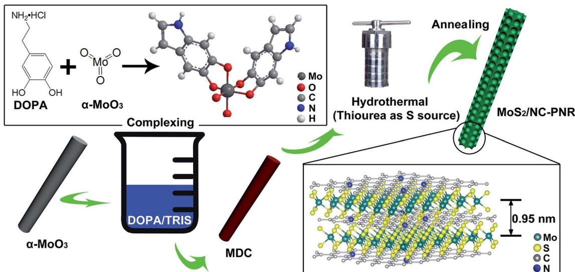
Fig. 2 Schematic illustration of MoS<sub>2</sub>/NC-PNR formation.
