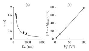
Fig. 5 (a) Measured relaxation times (dots) in PDMS films for varying applied voltages and frequencies as a function of initial surface separation  $D_0$ , compared to the model prediction  $\tau = \gamma/\kappa$  (solid line). (b) Measured displacement as a function of applied voltage  $V_0$ , for an initial distance  $D_0 = 3.93 \,\mu\text{m}$  and  $\nu_{AC} = 0 \,\text{s}^{-1}$ . The displacement scales with the square of the applied voltage.
