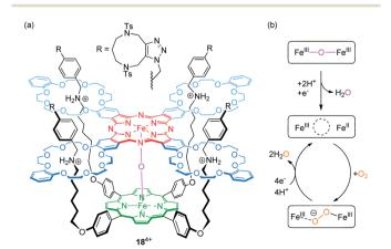
Fig. 15 (a) Structure of the fourfold threaded [2]rotaxane catalyst  $18^{4+}$ , which incorporates a  $\mu$ -oxo-dinuclear iron complex. (b) Suggested mechanism for the reduction of oxygen to water.
