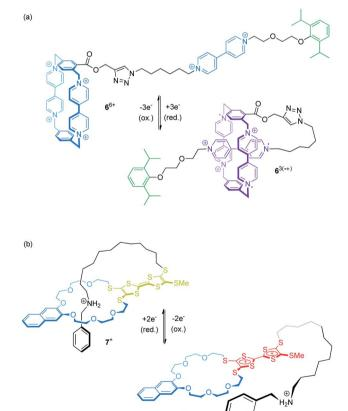
Fig. 7 Two examples for electrochemically controlled pseudo[1] rotaxanes which are convertible between a rope-like and a lasso-type conformation: (a) 66+ undergoes self-inclusion after reduction, whereas (b) 7<sup>+</sup> is preferentially threaded in the initial state and unthreads upon oxidation
