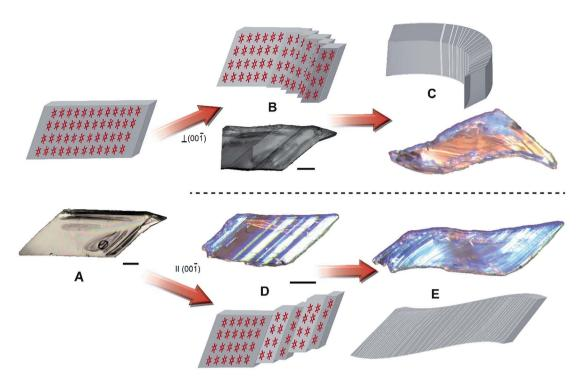
Fig. 4 Mechanical compliance of HMB crystals. (A) Optical image of a typical crystal, and molecular packing. HMB molecules are shown as sticks model (the bond radius is plotted as 0.2 Å) and the hydrogen atoms are omitted for clarity. (B-E) Optical images and cartoons of the evolution of twinned domains that evolve after force has been applied to the crystal normal (B and C) or parallel (D and E) to the  $(00\overline{1})$  plane. The length of the scale bars in all panels is 100 µm.
