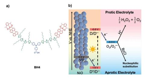
Scheme 1 (a) Molecular structure of BH4. (b) Schematic representation of the DSPEC for H<sub>2</sub>O<sub>2</sub> production in protic electrolyte and nucleophilic substitution in aprotic electrolyte.
