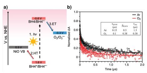
Fig. 4 (a) Energy diagram for charge transfer kinetics of BH4-sensitized NiO film. (b) Nanosecond TA spectra of BH4-sensitized NiO film at 615 nm in 0.1 M LiClO<sub>4</sub> inert electrolyte in acetonitrile, Ar (black trace) and O<sub>2</sub> (red trace). Excitation: 500 nm.
