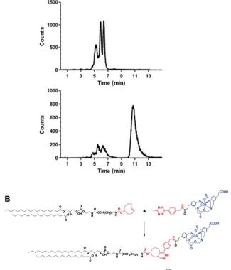
Fig. 4 (A) Radio-HPLC chromatograms of (top) [ $^{68}$ Ga]Ga-HBED-CC-tetrazine precursor and (bottom) reaction between 4 and 5, after 15 min at 60 °C. (B) Scheme of the reaction between TCO-modified PE (4) and [ $^{68}$ Ga]Ga-HBED-CC-tetrazine (5).
