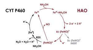
Fig. 2 Working mechanism for  $NH_2OH$  oxidation by heme P460 cofactors. The steps indicated in black distinguish cyt P460, in which the  $\{FeNO\}^6$  persists and can undergo nucleophilic attack by  $NH_2OH$ . In HAO, no  $\{FeNO\}^6$  has been observed, presumably due to facile release of NO, its stoichiometric product of  $NH_2OH$  oxidation. Adapted from ref. 23.
