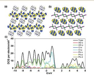
Fig. 3 Molecular orbitals of the HOMO (a) and LUMO (b) for OIHP-AD. (c) Total/partial electronic density of states (TDOS and PDOS) for the DFT optimized structure of OIHP-AD.
