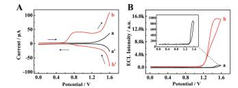
Fig. 5 (A) Differential pulse voltammetry (DPV) and (B) ECL-potential profiles of the TPE NCs modified GCE in (a) PBS solution and (b) PBS + 18 mM TEA solution.
