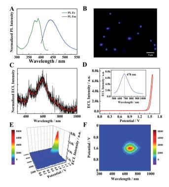
Fig. 3 (A) Normalized PL excitation spectra and PL emission spectra of TPE NCs in PBS solution. (B) Fluorescence microscopy image of TPE NCs. (C) The ECL spectra of individual TPE molecules in acetonitrile with TEA as a coreactant. (D) The ECL-potential curve of TPE NCs. The inset of (D) the 2D ECL spectra of TPE NCs in PBS solution with TEA as a coreactant. The ECL-potential-wavelength of TPE NCs via a 3D surface image (E) and 3D heat map image (F).
