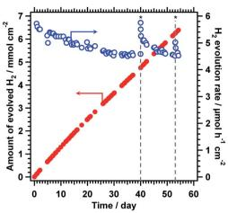
Fig. 4 Time course of water splitting activity of  $5 \times 5$  cm<sup>2</sup> TiO<sub>2</sub>/ CoOOH/RhCrOx/SrTiO3:Al sheet in panel reactor. Reaction conditions: photocatalyst, 20 mg; reaction solution, 1 mm deep distilled water; reaction temperature, 291 K; light source, AM 1.5G solar simulator. Asterisk symbols (\*) indicate interruption of the illumination for two days
