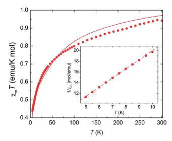
Fig. 2 Magnetic susceptibility of complex 1 as a function of temperature, plotted as  $\chi_m T$  vs. T (main panel) and  $1/\chi$  vs. T (inset). Dots: experimental data. Solid line: ligand-field calculation. Dashed line: Curie–Weiss fit.
