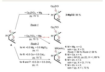
Scheme 2 Reductive metalation of A using  $Cp_2ZrCl_2/Mg$  ( $3 \cdot MgCl_2$ ) as well as  $Mg/MgCl_2$  (4),  $Ca/Cal_2$  (5),  $Zn/ZnCl_2$  (6) and  $Zn/Znl_2$  (7).
