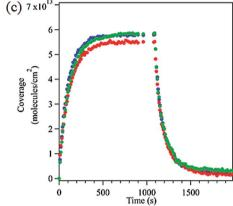
Fig. 1 (a) FTIR spectrum of limonene adsorbed on  $SiO_2$  surface at 22 mTorr equilibrium pressure (scale bar = 0.01 absorbance units). (b) Absorbance spectra in the C-H stretching region as a function of time during adsorption (blue) and desorption (red). (c) Temporal evolution of the adsorption and desorption of limonene on  $SiO_2$  (triplicate experiments are shown).
