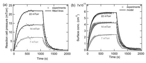
Fig. 5 (a) Temporal evolution of limonene pressures in the reaction cell and (b) adsorbed limonene concentrations on  $SiO_2$  as a function of time for three different limonene equilibrium pressures, 7 (light grey), 14 (dark grey) and 22 (black) mTorr. Error bars represent the standard deviation between triplicate replicates of the same experiment.
