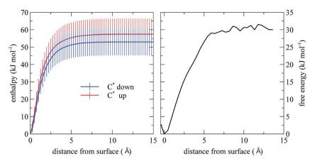
Fig. 3 Desorption enthalpy and free energy computed from MD simulation. The error bars are based on the standard deviation of the energy computed for the 100 initial structures.
