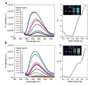
Fig. 5 Aggregation-induced emission effect of the TSCT-HABs. PL spectra and the relative emission intensity of Ac3TRZ3 (a) and TAc3TRZ3 (b) in THF/water mixed solvents at a concentration of  $1\times 10^{-5}$  mol L<sup>-1</sup>; inset: PL images with different water fractions ( $f_{\rm w}$ ) under UV light (365 nm).
