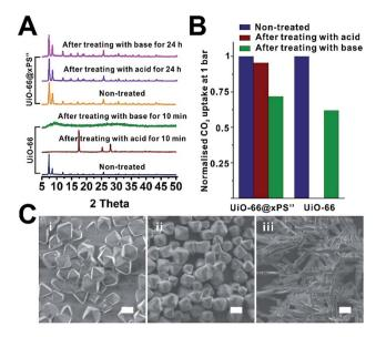
Fig. 6 PXRD patterns (A) and normalized CO $_2$  uptake at 195 K (B) of non-treated UiO-66 and UiO-66@xPS" and after treating them with 1 M H $_2$ SO $_4$  and 1 M NaOH at 50 °C for different times. (C) SEM images of UiO-66 (i), UiO-66@PS" after treating with 1 M H $_2$ SO $_4$  for 24 h (ii), and UiO-66 after treating with 1 M H $_2$ SO $_4$  for 10 min (iii); scale bars are 1  $\mu$ m for (i) and (ii), and 2  $\mu$ m for (iii).
