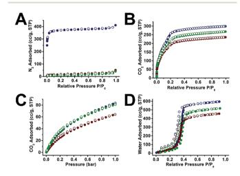
Fig. 4  $N_2$  sorption isotherms at 77 K (A),  $CO_2$  sorption isotherms at 195 K (B) and 273 K (C), and water vapor sorption isotherms at 298 K (D) of UiO-66 (navy), UiO-66@xPS (red) and UiO-66@xPBA (green). UiO-66@xPS and UiO-66@xPBA isotherms were normalized by subtracting the mass of the polymer (Table S5†).
