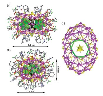
Fig. 1 (a) and (b) The X-ray crystal structure of Ag<sub>10</sub>@(Mo<sub>7</sub>O<sub>26</sub>)<sub>2</sub>@Ag<sub>70</sub> nanoclusters viewed along two orthogonal directions. The inner silver atoms of the  ${\rm Ag_{10}}$  kernel are highlighted in black.  ${\rm Mo_7O_{26}}^{10-}$  and  $MoO_4^{2-}$  are represented by green and yellow polyhedra, respectively. (c) The Ag<sub>70</sub>S<sub>36</sub> shell with silver heptagons highlighted in green.
