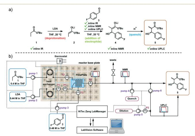
Fig. 1 a) Reaction scheme showing the deprotonation of tert-butyl propionate 1, its reaction with aldehyde electrophile 3, then quench to afford aldol product 5; b) schematic view of the final reaction setup used in this study, showing the placement of pumps, sensors (T = temperature sensor; P = pressure sensor) and PAT instruments, with their connection to the LabVision control system (black dotted line = electronic connection, blue dotted line = heat transfer fluid circulation).
