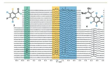
Fig. 3 Stacked NMR spectra of the reaction mixture, showing the extent of aldehyde 3 conversion to product enolate 4. These spectra were acquired using the Magritek Spinsolve Ultra 43 MHz equipped with glass flow-through cell.
