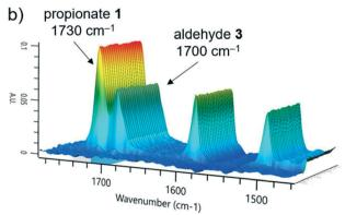
Fig. 2 Representative ReactIR spectra showing a) tert-butyl propionate starting material 1 and its deprotonation to form enolate 2; b) a combined solution of tert-butyl propionate 1 and aldehyde electrophile 3.
