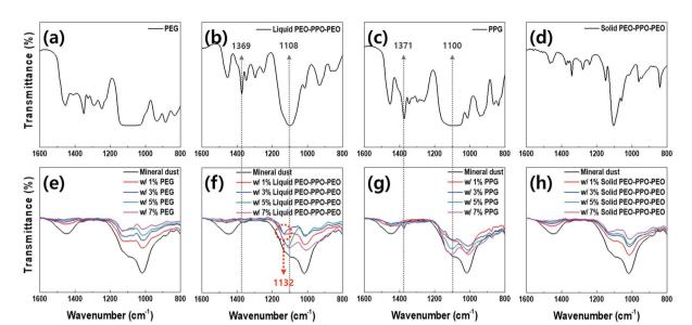
Fig. 3 ATR-FTIR spectrums of (a) liquid PEG, (b) liquid PEO-PPO-PEO, (c) liquid PPG and (d) solid PEO-PPO-PEO polymers and mineral dust mixed at 1:1 w/v ratio with polymer aqueous solutions of (e) liquid PEG (1-7 v/v%), (f) liquid PEO-PPO-PEO (1-7 v/v%), (g) liquid PPG (1-7 v/v%) and (h) solid PEO-PPO-PEO (1-7 w/v%). All samples were dried in electric oven at 50 °C for a week. The black solid lines in (e) – (h) represent the mineral particles treated by water alone
