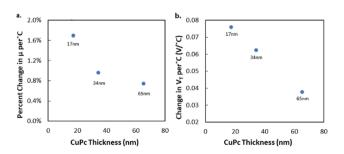
Fig. 4 Effect of CuPc thickness on BGBC OTFTs performance as a function of temperature (between 25 °C and 85 °C for air and 20 °C to 150 °C for vacuum). (a) % change in hole mobility,  $\mu_{\rm H}$  compared to baseline at 25 °C per °C and (b) the change in threshold voltage  $V_{\rm T}$  per °C.
