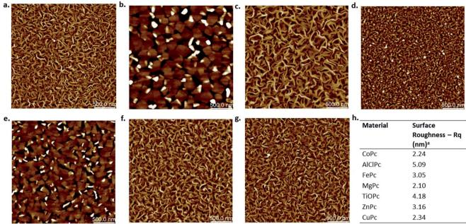
Fig. 5 AFM images (2.5  $\mu$ m  $\times$  2.5  $\mu$ m) of (a) CoPc (b) AlClPc (c) FePc (d) MgPc (e) TiOPc (f) ZnPc (g) CuPc deposited on heated silicon substrates (T = 140 °C) under vacuum (h) surface roughness values (nm) for each film.
