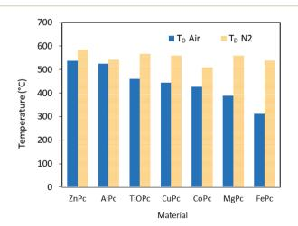
Fig. 6  $T_{\rm D}$  of MPcs in air (blue) or nitrogen (yellow horizontal lines). These temperatures were found from 5% mass degradation during TGA.
