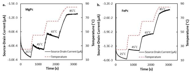
Fig. 7 Current response to temperature changes at constant voltages, with  $V_{SD} = -50$  V. (a) MgPc BCBG devices,  $V_{GS} = -30$  V and (b) FePc devices,  $V_{GS} = -60$  V, were held at a constant bias while the  $I_{SD}$  was measured. The devices began testing at T = 25 °C and the temperature was increased at regular timepoints up to 85 °C in vacuum.
