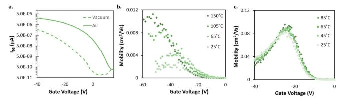
Fig. 2 Characterization of AlClPc OTFTs. (a) Transfer curves for AlClPc BGBC devices deposited at  $T = 140 \,^{\circ}$ C, and tested in air ( $V_{SD} = -50 \,^{\circ}$ V), and vacuum, at T = 25 °C.  $V_{GS}$  vs.  $\mu_{H}$  curves at temperatures ranging from 25 °C to 150 °C in vacuum (b) and temperatures from 25 °C to 85 °C in air (c).
