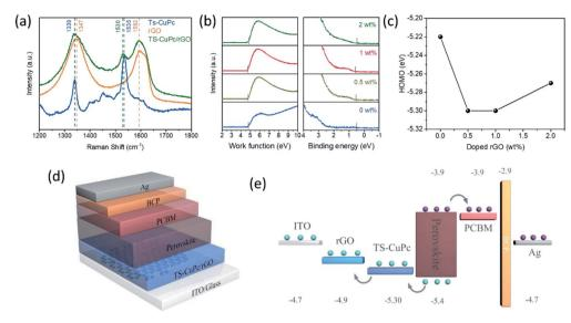
Fig. 3 (a) Raman spectra of rGO, TS-CuPc, and TS-CuPc/rGO thin films. (b) Ultraviolet photoelectron spectra (He I: 21.2 eV) of the TS-CuPc thin films with different doped rGO concentrations. (c) Dependence of HOMO level on the concentration of doped rGO. (d and e) Device architecture and the schematic energy structure of photodetectors with TS-CuPc/rGO as the HTL.
