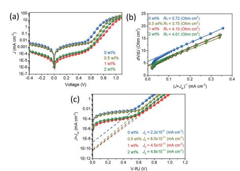
Fig. 4 (a) Dark current density–voltage curves of photodetectors with different rGO concentrations. (b) Calculated  $R_s$  of devices by plotting dV/dJ versus  $(J + J_{SC})^{-1}$ . (c) Dark saturation current density  $(J_0)$  for devices is calculated from the plot of  $\ln(J + J_{SC})$  versus (V + RJ).
