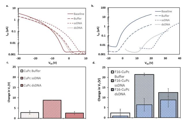
Fig. 6 Transfer curves (a and b) and absolute change in threshold voltage (c and d) of  $1 \,\mu\text{L}$  of  $1 \,\mu\text{M}$  ssDNA,  $1 \,\mu\text{M}$  dsDNA or buffer were added to baseline of CuPc OTFT (a and c) and  $F_{16}$ -CuPc (b and d). All characterization was performed at  $51.1 \,^{\circ}\text{C}$  in air except for the superimposed inner bars in (d) (filled blue rectangle) which were characterized at  $25.0 \,^{\circ}\text{C}$ .
