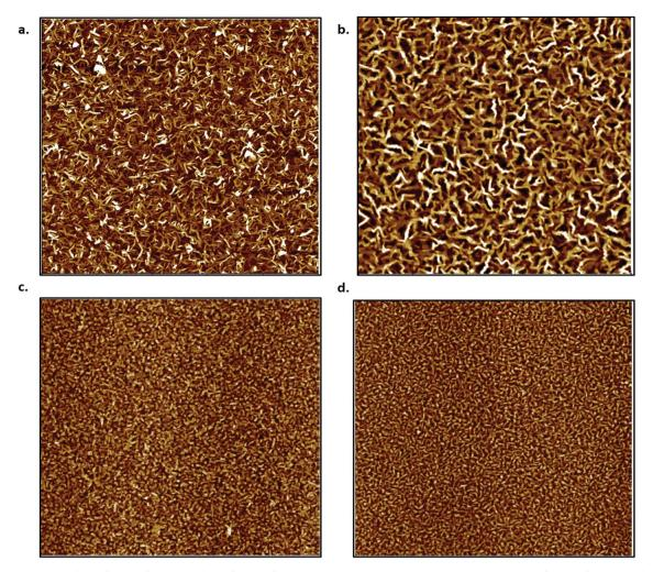
Fig. 5 AFM images of CuPc (a and c) and F<sub>16</sub>-CuPc (b and d) thin films deposited on SiO<sub>2</sub> substrates at 140 °C (a and b) and 20 °C (c and d). Images (a and b) are 5  $\mu$ m imes 5  $\mu$ m while (c and d) are 2.5  $\mu$ m imes 2.5  $\mu$ m.
