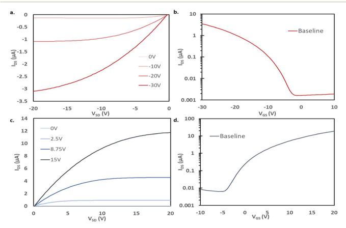
Fig. 2 Output and transfer curves for baseline BGBC OTFTs tested at 25  $^{\circ}$ C. (a) Output curve and (b) transfer curve ( $V_{DS} = -20$  V) for CuPc devices. (c) Output curve and (d) transfer curve ( $V_{DS} = 20 \text{ V}$ ) for  $F_{16}$ -CuPc devices.
