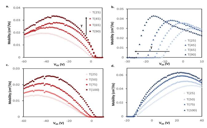
Fig. 3 Field-effect mobility for (a and c) CuPc and (b and d)  $F_{16}$ -CuPc BGBC devices deposited at T = 140 °C with respect to applied gate-source voltage ( $V_{GS}$ ) for characteristic devices at varied temperatures in air (a and b) and vacuum (c and d). This mobility was calculated between adjacent points in the transfer data using eqn (2). Devices were tested in the range of T = 25 °C to T = 90 °C in air, and T = 25 °C to T = 100 °C in vacuum.
