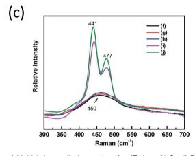
Fig. 11 (a) Initial charge discharge plot of an IT planar NaS cell. Raman spectra of the IT NaS battery cathode during the first discharge (b) and charge (c) at a current density of  $0.33~\text{mA}~\text{cm}^{-2}$ . The diagram is adapted/reproduced from ref. 28 with permission from the *Royal Society of Chemistry*.
