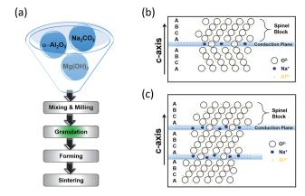
Fig. 5 (a) Conventional tube ( $\beta''-Al_2O_3$ ) production process. Crystal structure of (b)  $\beta-Al_2O_3$  and (c)  $\beta''-Al_2O_3$ . The diagram is adapted/reproduced from ref. 67 with permission from *Elsevier*.
