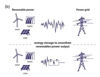
Fig. 1 (a) Energy shift from solar power using battery storage. (b) Energy storage provides stored electricity to the grid and stable power output from renewable sources smoothening.
