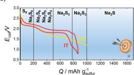
Fig. 12 (a) Graphical representation of the colour of different sodium polysulfides when dissolved in TEGDME. (b) Initial charge–discharge curves of a NaS battery at IT and RT. The diagram is adapted/reproduced from ref. 30 with permission of the *Royal Society of Chemistry* and from ref. 212 with permission of *John Wiley and Sons*.
