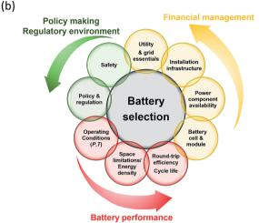
Fig. 2 (a) Current status of Battery Energy Storage Technologies (BESS). Data taken from ref. 17 and 18. Metal air batteries: Zn-air and Li-air; RFB: Zn-Ir, Zn-Br<sub>2</sub>, Zn-NiO, Ir-Cr, VRFB. Pb-acid batteries: advanced and valve-regulated. Li based batteries: LTO, LCO, LFP, NMC, NCA and Li-polymer. Ni based batteries: Ni-Cd, Ni-Fe. (b) Criteria for BESS selection.
