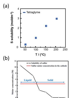
Fig. 13 (a) Solubility of sulfur in TEGDME at the IT range. The diagram is adapted/reproduced from ref. 28 with permission from the *Royal Society of Chemistry*. (b) Relationship between the solubility of sulfur depending on  $Na_2S_x$  (x=1-8) and the sulfur cathode. The molar concentration of sulfur in the cathode is calculated as the sum of liquid electrolyte and sulfur mass in the cathode. The diagram is adapted/reproduced from ref. 209 with permission from the *Electrochemical Society*.
