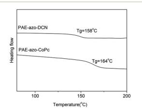
Fig. 5 DSC curves of PAE-azo-DCN and PAE-azo-CoPc.
